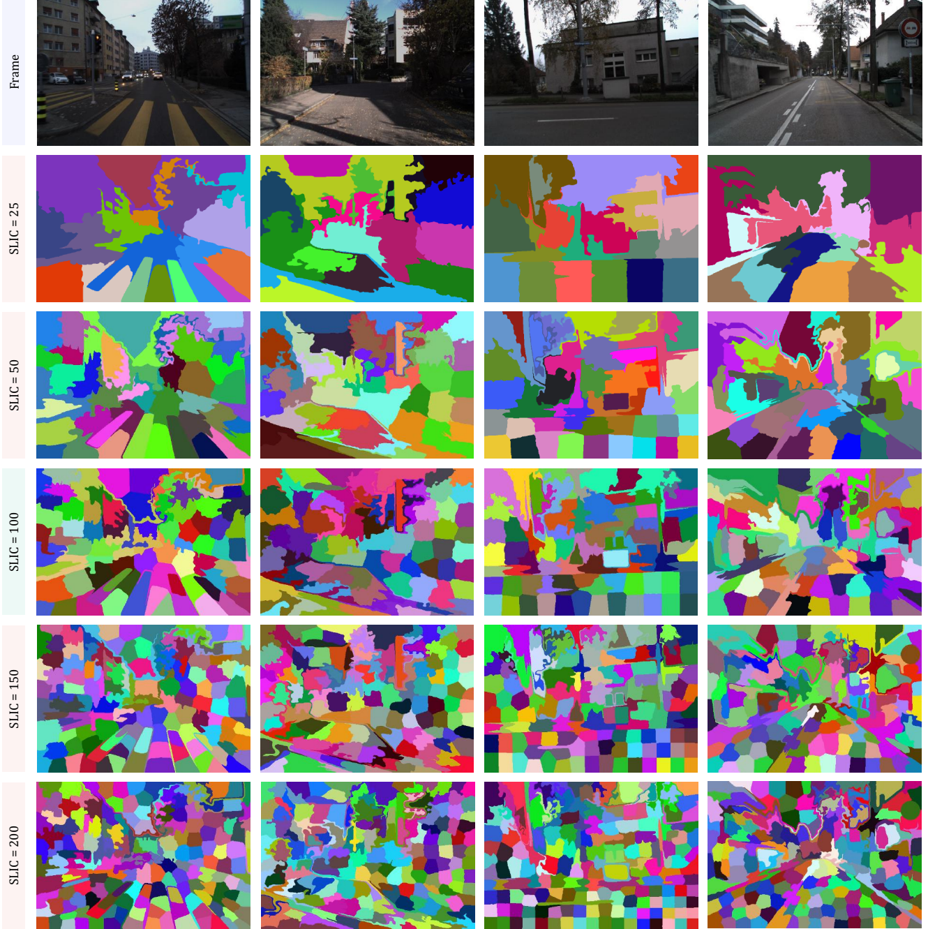
Figure 9. Examples of superpixels generated by SLIC [1] with different numbers of superpixels M_{sluc} (25, 50, 100, 150, and 200). Each colored patch represents one distinct and semantically coherent superpixel. Best viewed in colors.
